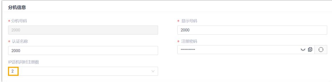
The screenshot shows the 'Phone Number' configuration page. The 'Number of simultaneous registrations for IP phones' dropdown is highlighted with a yellow box and set to the value '2'.
