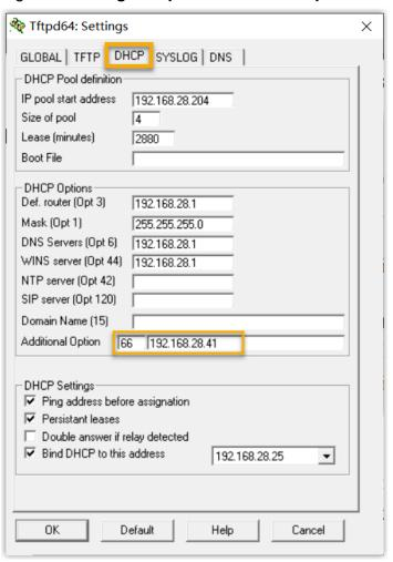
Figure 9. Configure option 66 on the Tftpd64's DHCP server
