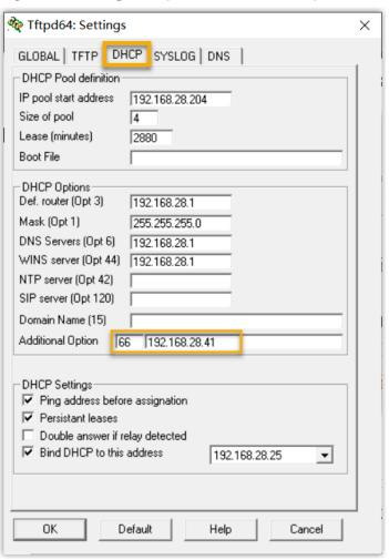
Figure 7. Configure option 66 on the Tftpd64's DHCP server
