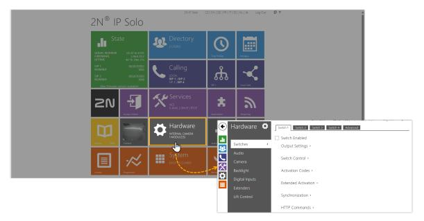
2. Under the **Switch 1** tab, configure the DTMF code for door release.
