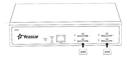
2. Press the SIM card to remove the SIM card.
