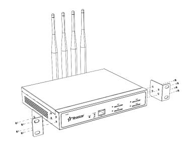
**2.** Place the TG gateway in the 19-inch rack and fix both brackets to the rack with the rack's proprietary mounting equipment.
