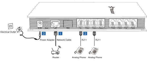
1. Connect TA gateway to the Internet LAN port can be connected to router or PBX.
